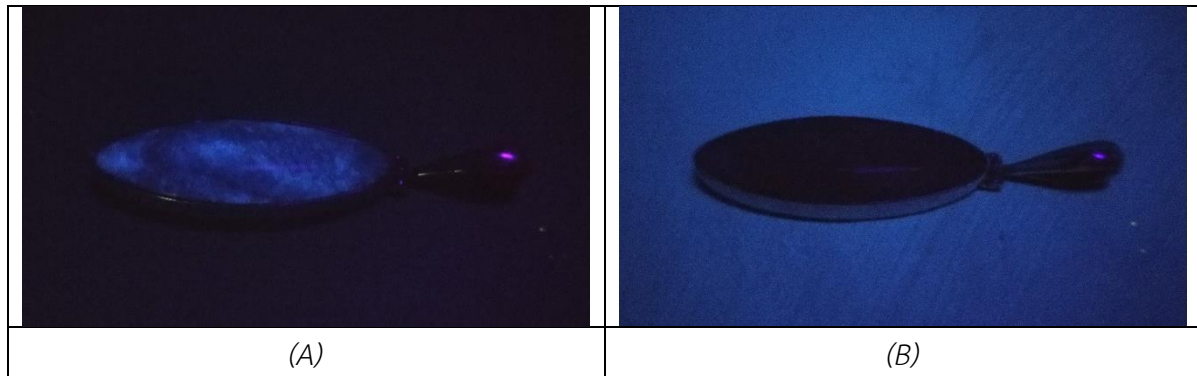
Figure 3: The stone in UV radiation: the white mineral grains fluoresce moderately chalky blue while the blue mineral grains show weakly chalky blue in LWUV (A), and the stone is inert in SWUV (B), Photos by B. Srisataporn
