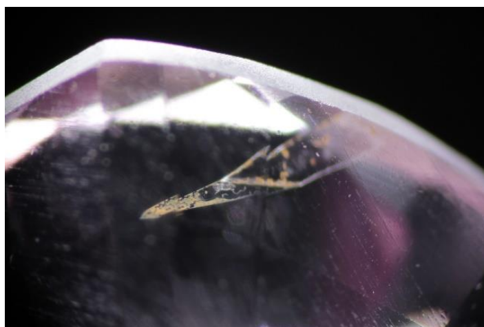
Figure 2(c): Iron stain in fracture. Photomicrograph by S.Saengbuangamlam; magnified 50x
