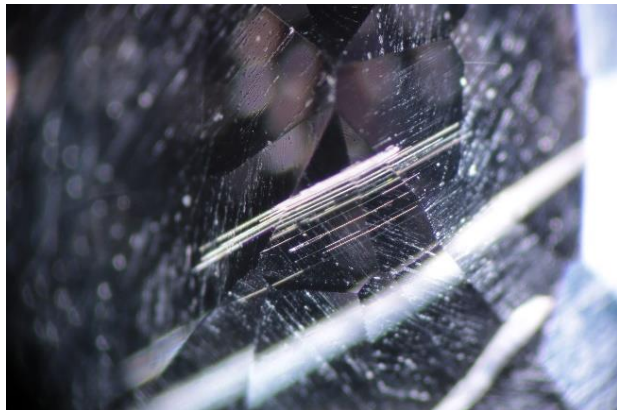
Figure 2(a): Parallel needle inclusion. Photomicrograph by S.Saengbuangamlam; magnified 50x
