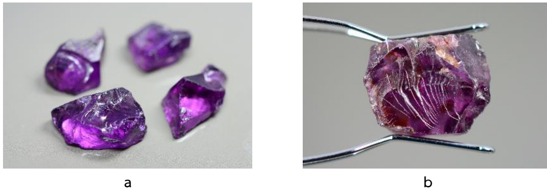
Figure 3: The rough samples show sub-angular shape (a) and conchoidal fracture (b).
