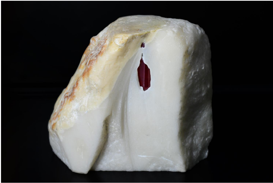
Figure 1: Rough “Ruby-in-marble” specimen showing a dark red crystal in white marble submitted to GIT-GTL for testing. Photo by S. Promwongnan.
