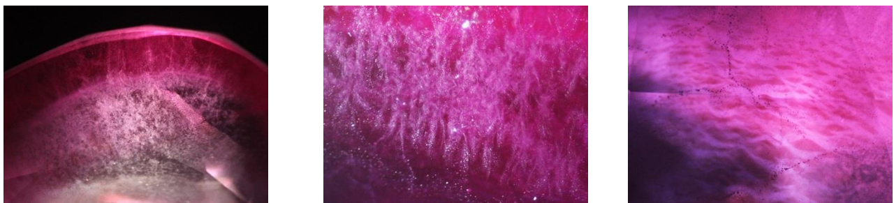
Figure 4: The thick red overgrowth layer is clearly seen on the pavilion side of the stone (left, magnified 16X). Higher magnification of the overgrowth layer revealed numerous fine wispy veil-like flux inclusions (center, magnified 25X) and
