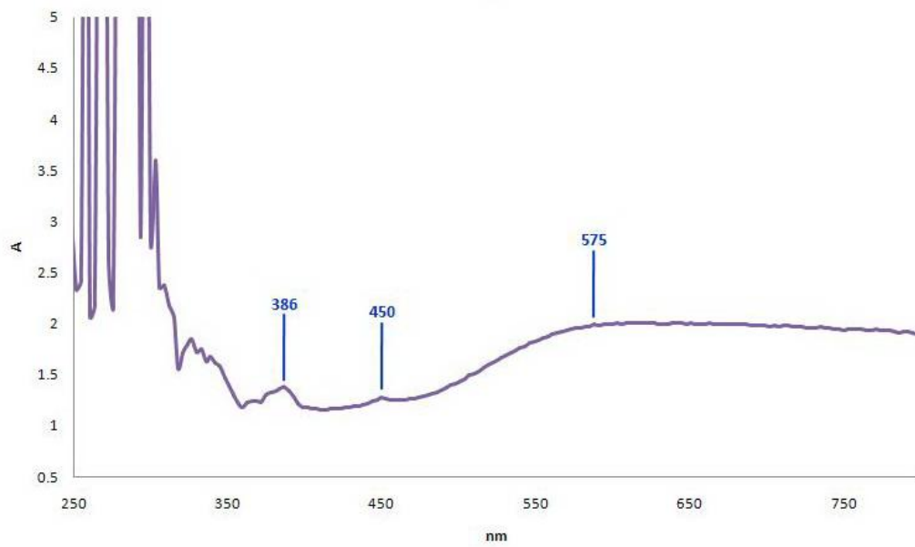
Figure 6: A representative non-polarized UV-Vis spectrum of the stone showing small Fe-related absorption peaks at 377/387 and 450 nm and dominant Fe 2+ /Ti 4+ IVCT absorption band maximized at around 575 nm.
