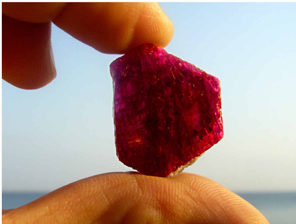
Figure 5: Sample of material that can be used for lead-glass fracture-filled treatment. Photo: Chakkaphan Sutthirat
